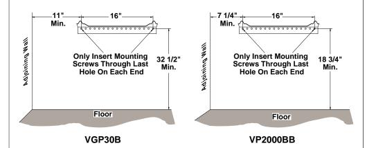
Figure 7 - Mounting Bracket Clearances
